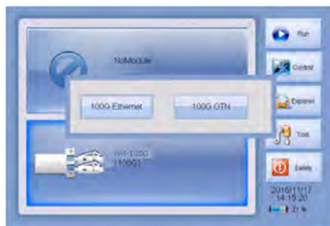
Figure 6.2 Select Test Application
