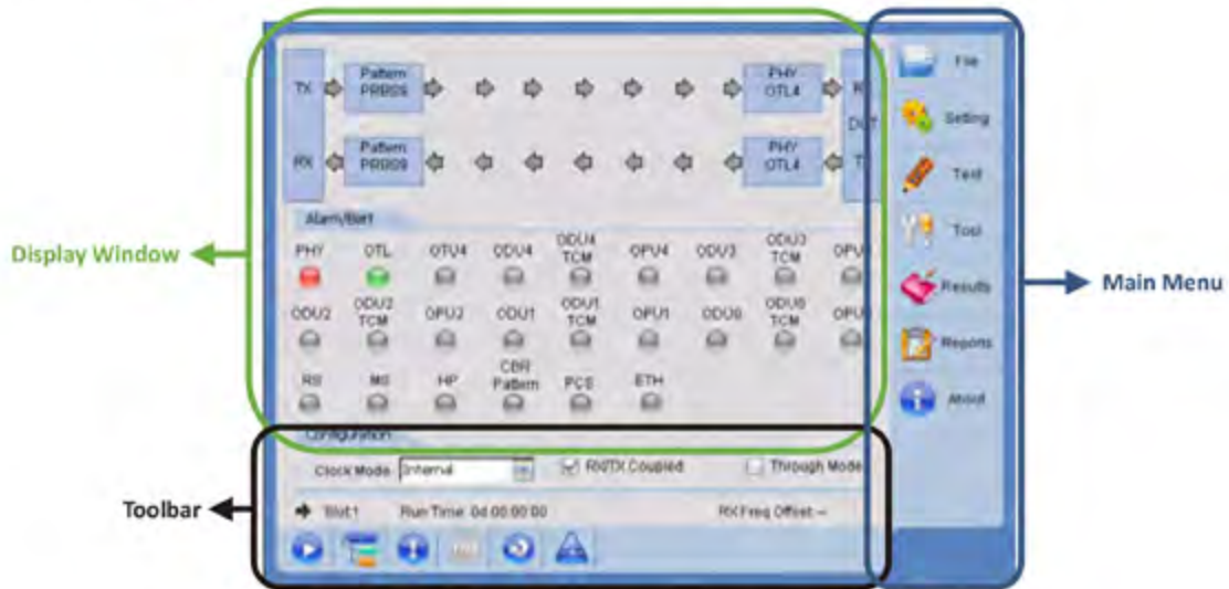
Figure 6.21 Main Interface of 100G OTN Application
