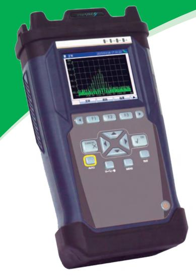
IVR-6123-OSA optical DWDM channel monitor is compact and low-cost test alternative solution to optical spectrum analyzers form DWDM system. IVR-6121-OSA is developed to measure exact power, frecuency, ONSR adaptable to DWDM network conditions. Information can be displayed in a graphic or table of results so that users can easily check the performance of each channel. It is ideal for the field application like installation, maintenance and upgrades for DWDM systems.
