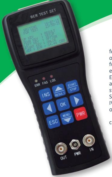
IVR-E1-2048 is a handheld E1 tester for analyzing error code performance of digital channels. It features complete functions and simple operation. It analyzes error codes of transparent E1, E1 FRAMED, E1 ONLINE, and optionally can analyze asynchronous RS232, synchronous RS232, synchronous V.35, V.35 FRAMED, and Synchronous TTL level interfaces. The IVR-E1-2048 can measure the frequency of input digital signals.
