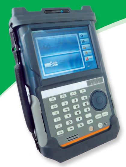
IVR-Sync Synchronisation Analyser is specially designed for conducting clock synchronisation of PTN or Packet Ethernet. It is developed in accordance with IEEE1588v2, SyncE, 1PPS+ToD, Ethernet, and E1 such standards, provides a complete clock, frequency, and time synchronisation test solution for operators.
