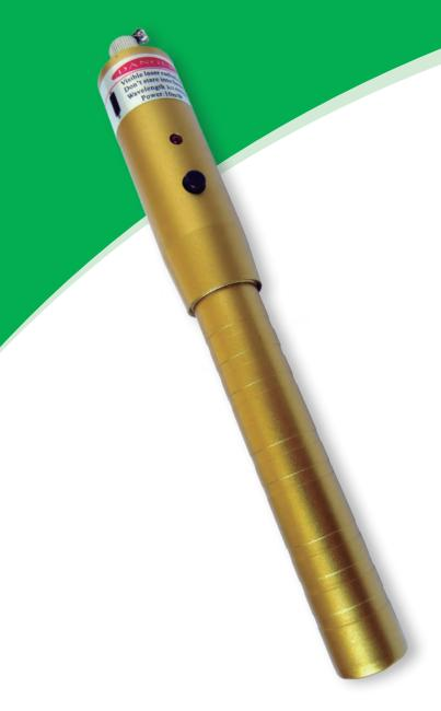
The IVR pen style VFL is specially designed for field personnel who needs a portable light source tool for fiber tracing, fiber routing, continuity testing, to locate breakpoints (bending or cracking in fiber optic cables), and poor connections. The IVR VFL works in an OTDR dead zone and is used for end-to-end visual fiber identification.
