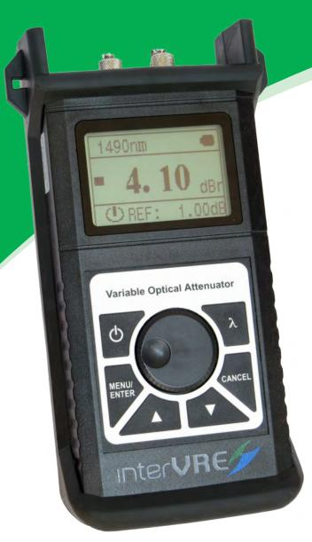
IVR-VOA handheld variable optical attenuator is used for continuously change the attenuation value of an optical signal. As the attenuator is used in the laser system for the on-line testing, it can be used in the digital system of communication devices such as DWDM, CWDM, Ethernet, SHD, PDH, OTN, CATV, and others.
